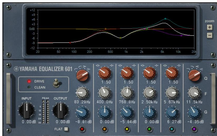
Equalizer 601 emulates the distortion characteristics of analog equalizers as used in the seventies. It provides musical-sounding drive and saturation.
