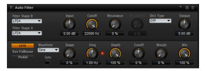
The morphing between the two shapes, as well as the cutoff, can be controlled with a manual pedal control, an LFO, or an envelope shaper.
