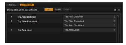
With the tabs at the top, you can specify whether you want to show the automation parameters for the slot, the global parameters, or all automation parameters.
