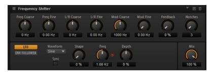
Unlike pitch shifters, where the frequencies are shifted by a factor, and where the harmonic relations are kept, a frequency shifter alters the harmonic relations. Therefore, a larger frequency shift usually results in a disharmonic sound.
