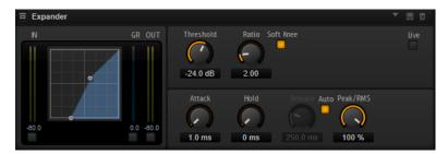
The graphical control to the left shows the expansion curve. You can edit the **Threshold** and **Ratio** values with the handles of this control. The input and output meters indicate the level before and after the expansion. The Gain Reduction meter indicates the current attenuation of the level.
