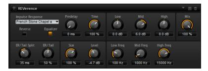
By recording an impulse in a room, you capture the characteristics of this room. Convolution superimposes these characteristics to the sound. The result is a very natural sounding reverb. Included with this effect is a collection of high-quality reverb impulse responses.
