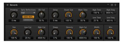
The early reflections are responsible for the spatial impression in the first milliseconds of the reverb. For emulating different rooms, you can choose between different early reflection patterns and adjust their size. The reverb tail, or late reverberation, offers parameters for controlling the room size and the reverb time. You can adjust the reverb time individually in three frequency bands.
