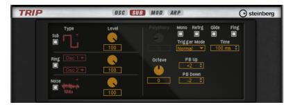
To activate the sub oscillator, the ring modulator, and the noise generator, click their **On/Off** buttons.
